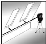
Reference for dormer installation
